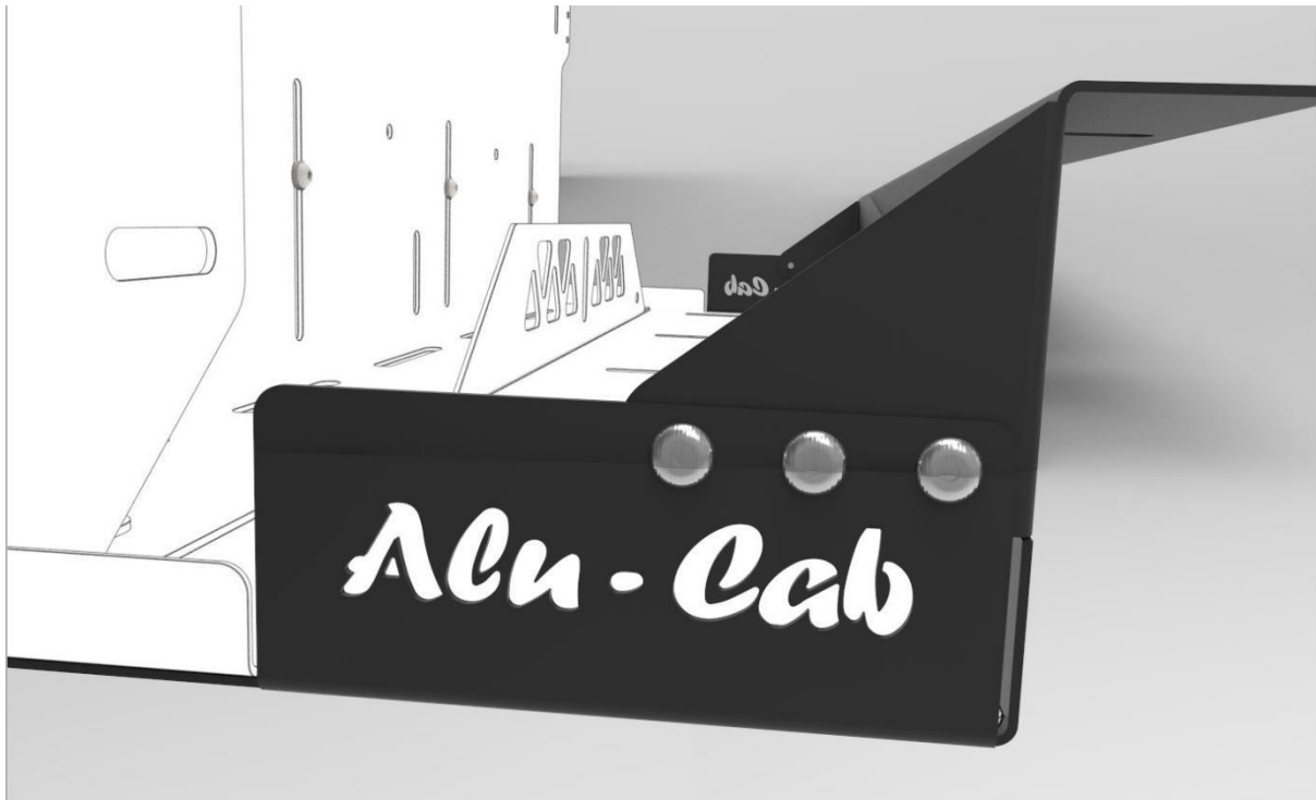
Figure 34: Side gussets for Shelf Mount Bracket
