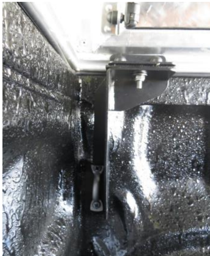
Figure 21: Front-Right Support Bracket Installed
